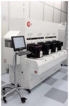
RECIF new 300mm G5+ platform installed in the clean room of (imec
