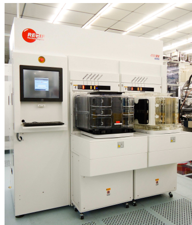
RECIF 450mm equipment installed in imec clean room
